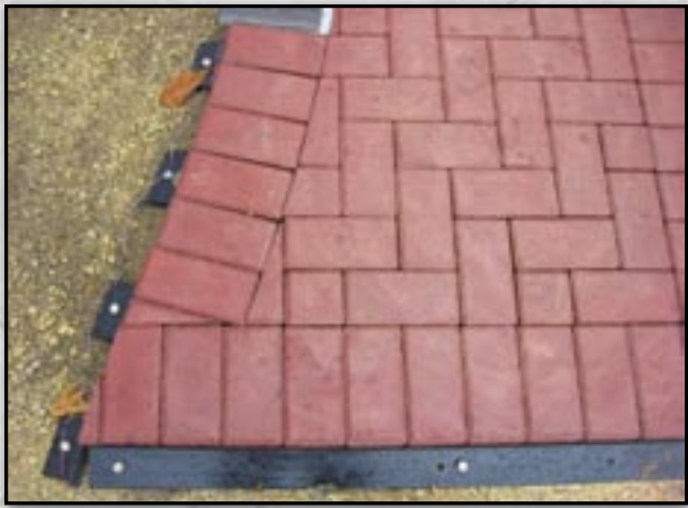
EDGING D - Manufacturer's and Test recommended spike spacing are the same.
