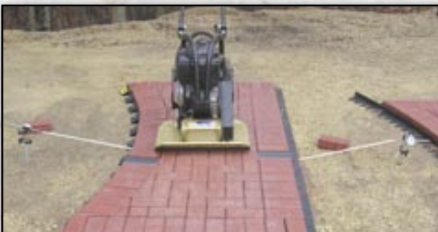
Deflection measurement was taken midway between spikes.
