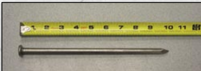
10" x \frac{3}{8} " steel spike used to spike edging.
