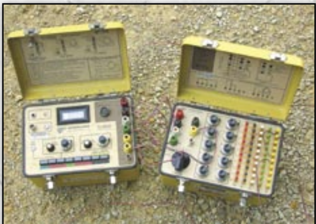
Testing equipment for data recording load sensing steel pavers.
