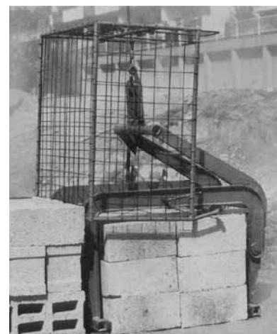
*The „Polyp 64“ mechanical grab for tower crane operation in use*
